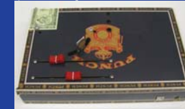
Figure 8. Next generation of cigar box ("frictionless" model) incorporates flat voice coil motors acquired from computer hard drives.
