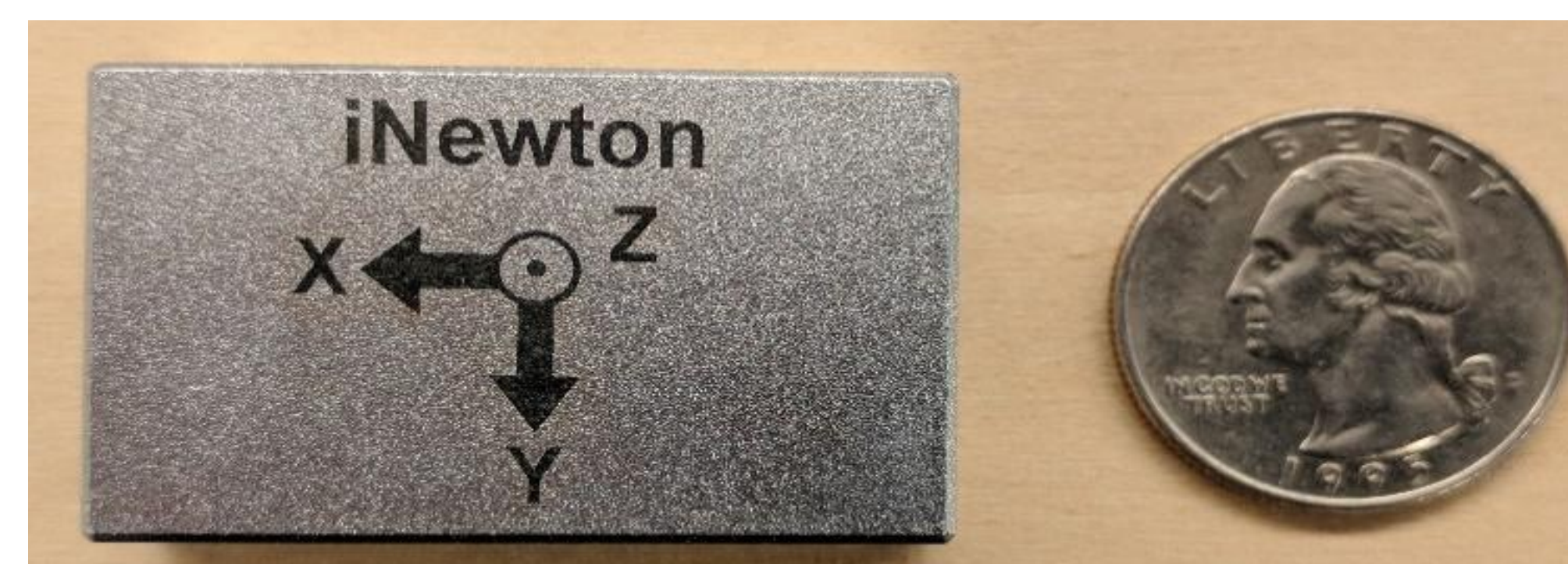
Figure 1: An iNewton with sensor-fixed frame of reference etched on top. It contains a triaxial accelerometer and angular rate gyro, which measure linear acceleration and angular velocity, respectively.
