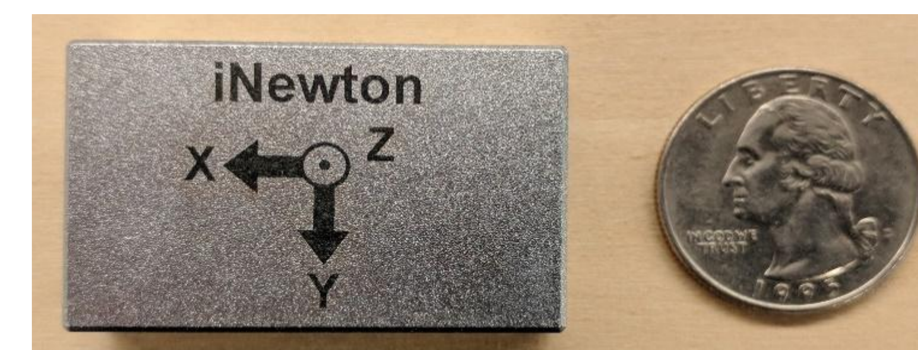
Figure 1: An iNewton with the sensor-fixed frame of reference etched on top. It contains a triaxial accelerometer and angular rate gyro, which measure linear acceleration and angular velocity, respectively.
